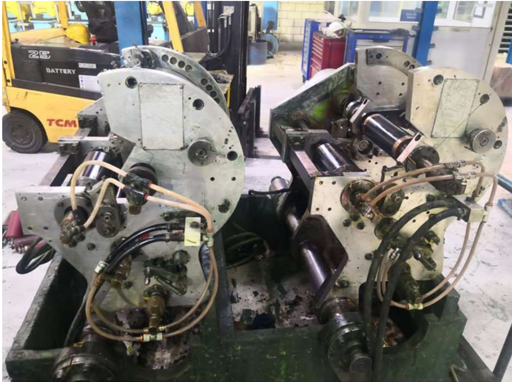
Inkers tripped and cleaned Machine stripped ready for moving
